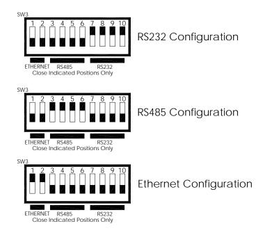
Figure 8-1: Com Configuration Jumper Settings (SW2)
